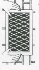
Using a wire which will pass through the screen, test for freedom of movement of the louvers to be sure there is no binding.
